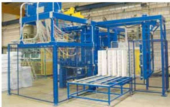
Picture 1 – HEITZ HBB 1412: Moulding machine with handling robot and stacking table. For the production of ICF elements with sheet metal or plastic connecting inserts, 3 elements per cycle.
