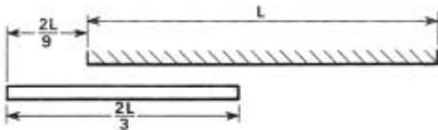
If the bore length is L then the stone length will not exceed  $\frac{2}{3}$ . To produce a parallel hole the stone must pass out of each end of the bore by one third of its own length i.e.  $\frac{1}{3}$ .
