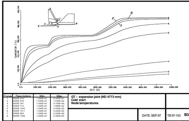
Fig. 8 Node temperatures of strutral points
