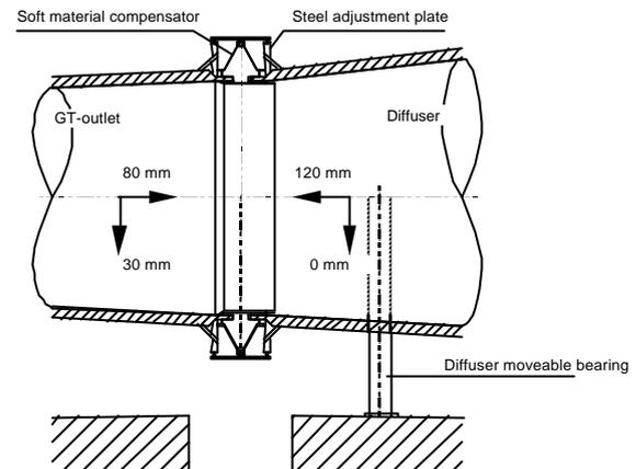
Fig. 2 Installation of fabric expansion joint
