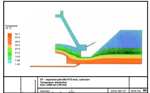
Fig. 11 Temperature map where T=140min
