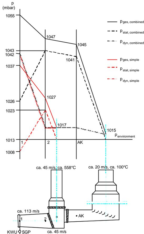
Fig. 20 Pressure pattern of exhaust gas section
