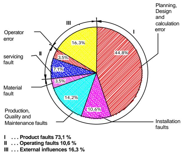
Fig. 6 Distribution of the primary causes of damage to industrial gas turbines according to installation, warranty and maintenance
