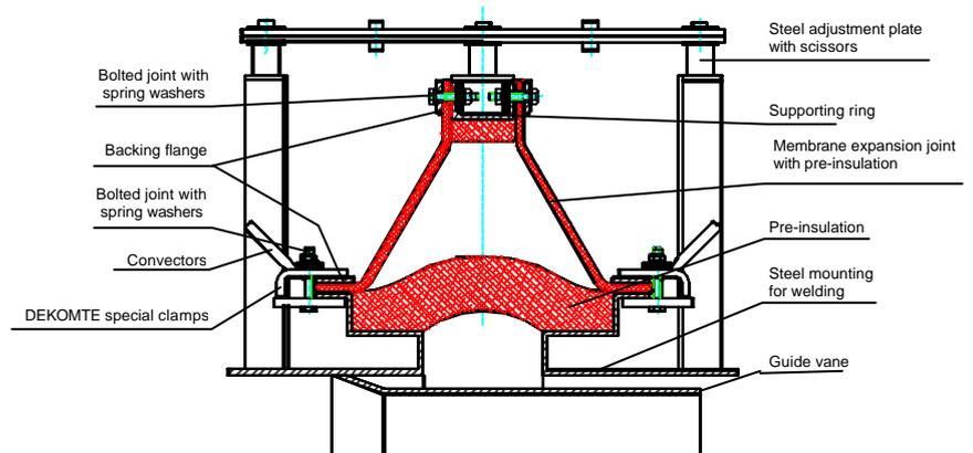
Fig. 4 DEKOMTE membrane expansion joint
