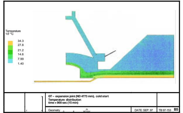
Fig. 9 Temperature map where T=15min
