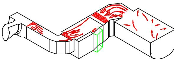
Fig. 18 Illustration of flow, section through the gas turbine system
