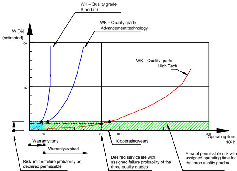
Fig. 5 Failure probability curve
