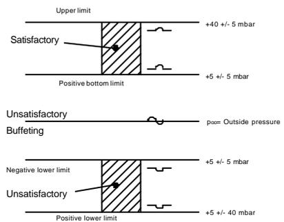
Pressure conditions on expansion joint at different static pressures with superimposed pressure pulses of  $\pm 5 \text{ mbar illeg}$ .
