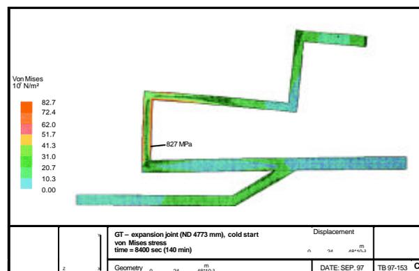
Fig. 12 Comparison stresses where T=140min
