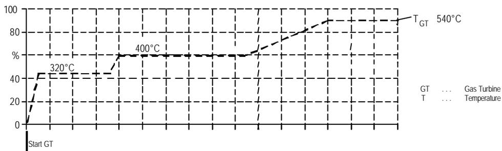
Fig. 7 Cold start for GT operation on natural gas
