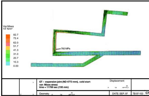
Fig. 14 Comparison stresses where T=195min
