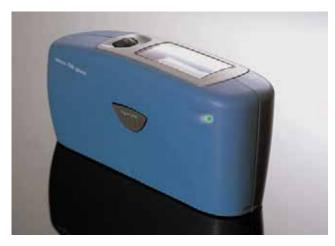
In order to obtain differences clearly over the whole range from matte to high gloss, three measurement geometries were specified in international standards. Each geometry is optimized for a specific gloss range.
