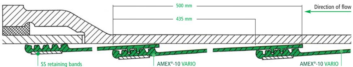
The AMEX<sup>®</sup>-10 VARIO Seal bases on the principle of the AMEX<sup>®</sup>-10 MONO Seal. Numberless VARIO Seals can be connected to an endless unit by choice. Each AMEX<sup>®</sup>-10 VARIO Seal is geared and secured to the next seal, this avoiding a replacement and sliding.
