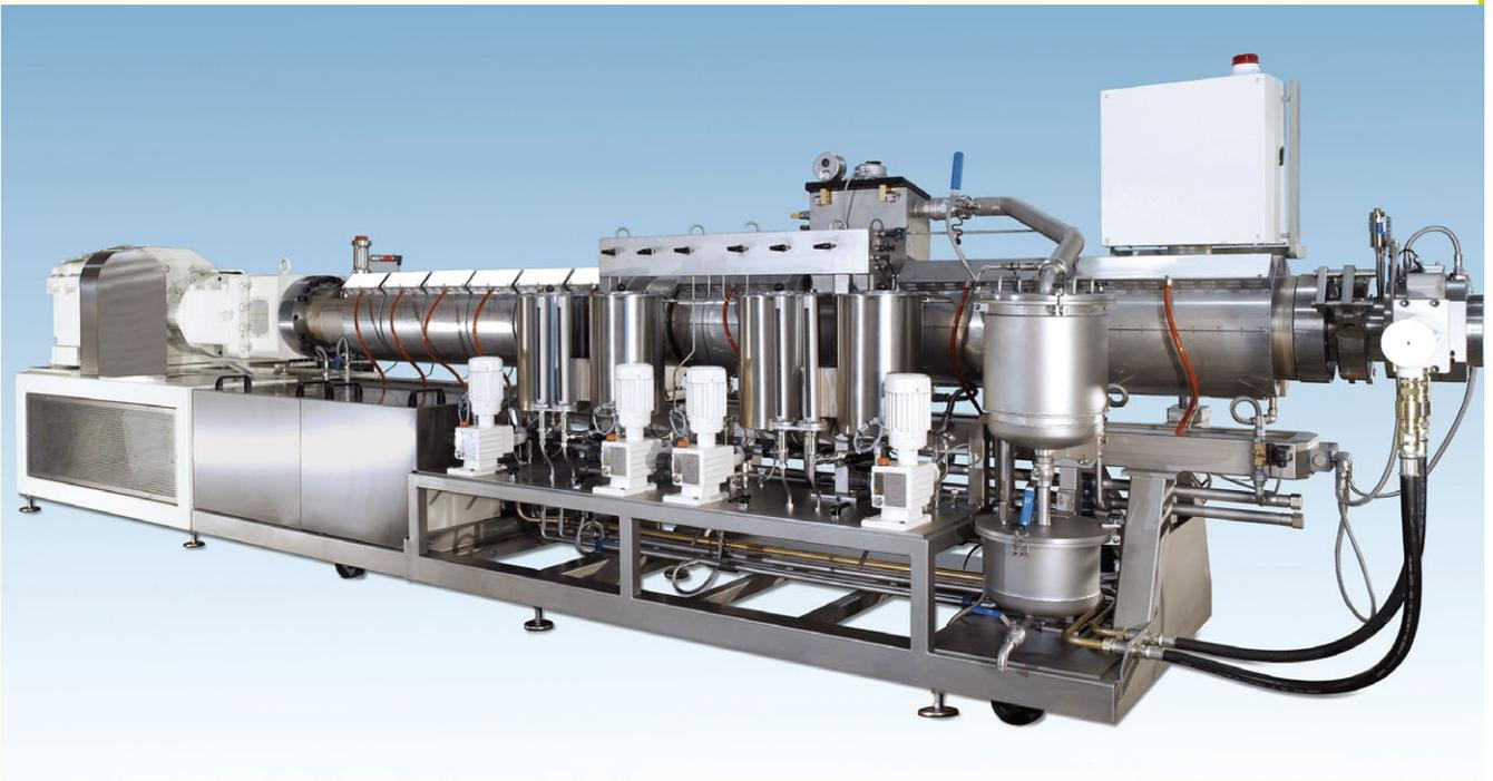
**Continuous production: mixing, cooking, forming, cooling and cutting**
