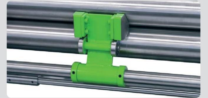
**Cone bending attachment with trailing shoe**
