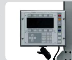
The program consists of sections, where each section is provided with a bending value. This enables easy and quick programming of the machine for different bending operations. The CNC system can operate with "interpolation", where the rolls are adjusted simultaneously with the feeding operation.
