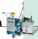
With the development of the mortar applying machine, MAM, LISSMAC is reacting to the market's increased demands for quicker and cheaper building work. The machine lays an exact mortar joint with high precision to be able to eliminate any needs for levelling out during the wall is erected with thin bed mortar.
