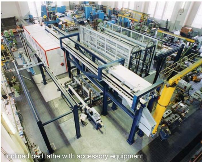
Inclined bed lathe with accessory equipment
