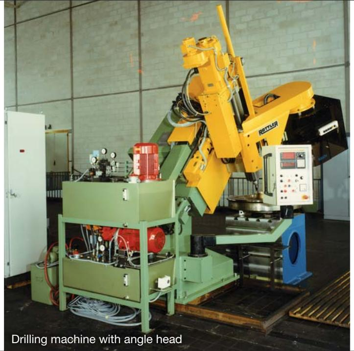
Drilling machine with angle head
