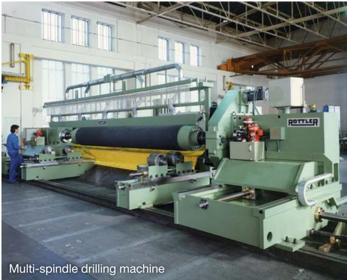
Multi-spindle drilling machine
