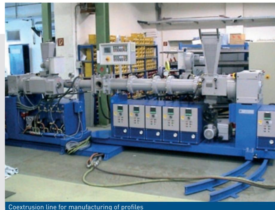
Coextrusion line for manufacturing of profiles
