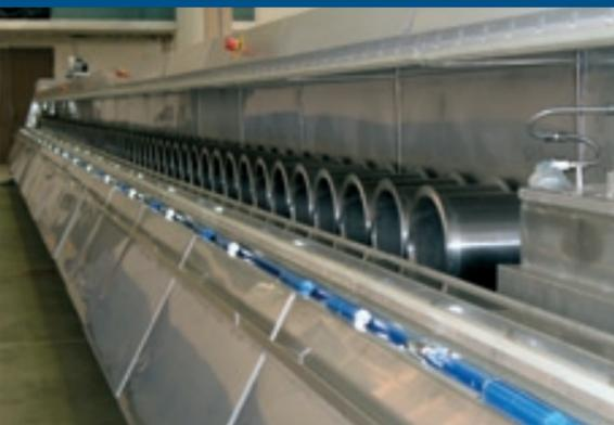
LCM 20 RS/EL Dipping roller section
