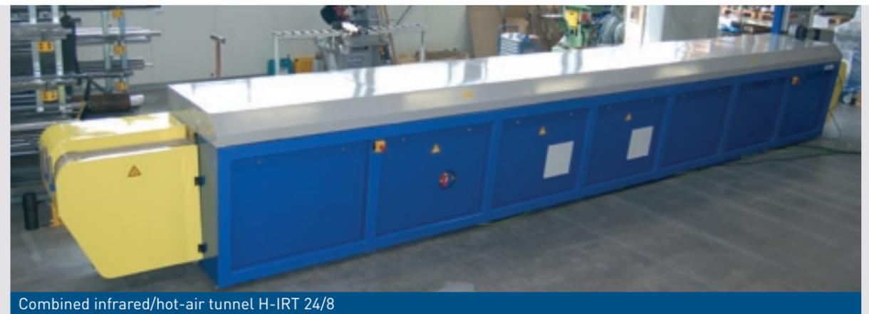
Combined infrared/hot-air tunnel H-IRT 24/8
