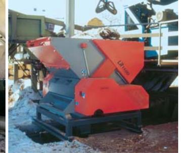
**Shredding of joinery workshop waste to generate heat for the heating of buildings**
