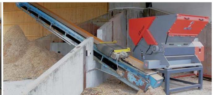
**Shredding of a door manufacturer's production waste to generate heat in a CHP plant**
