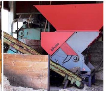
**Shredding of a stair builder's waste; shredded material used to generate heat for the heating of buildings**
