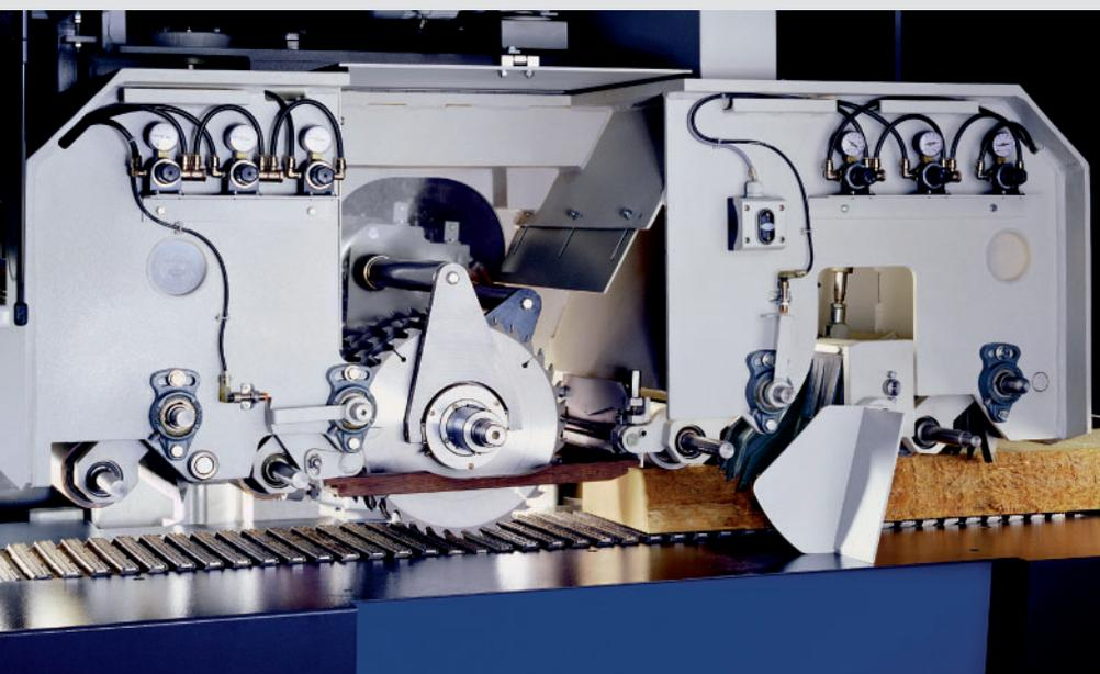
A strong production platform, whether as a gang rip saw or an optimizing rip saw. A well-equipped basic machine as standard, with many intelligent options. Robust construction and a solid pressure unit are the foundation for best possible material transport and cutting quality. With the right blades you can achieve a glue-joint quality cut right here at the rip saw. These extraordinarily strong machines can handle the toughest material. Even thickness variances in the material are no problem.
