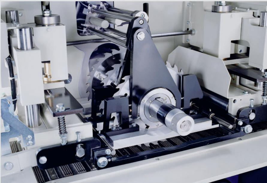
The moving pressure shoe segments, synchronous with the moving blades, ensure superior board control during the cutting process. Even outer edges are securely held down during ripping and transported safely out of the machine. Ripped pieces cannot lift up, so throughput is not interrupted. Optimal material hold-down means better quality of cut.
