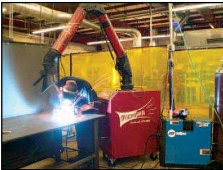
TM1000 Portable Collector in Weld Cell
