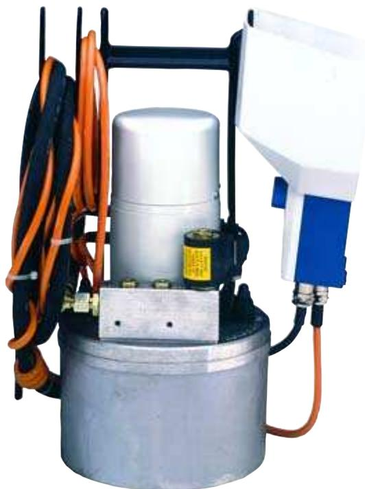
For all applications on site and regular workload in fabricating the HA 1-ES is our standard power pack. Through a combined safety and return valve, an overload of either the power pack or the connected tool is prevented. Userfriendly operation by foot-switch with integrated emergency button and integrated 24 V controls for hand-operated tools meets the latest safety regulation VVA/UVB.
