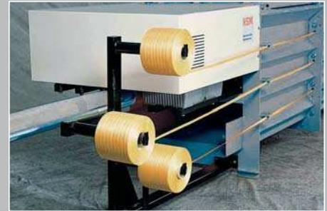
Bales are strapped easily and tightly with polyester tape through the use of proven strapping equipment.
