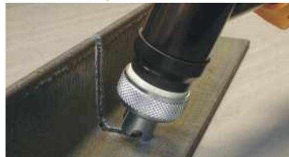
Extended consumables for cutting at inaccessible parts of workpiece
