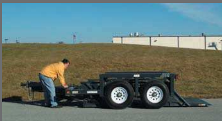
Lower entire deck to ground level
