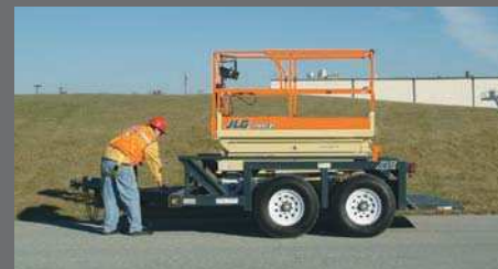
Lift to transport position
