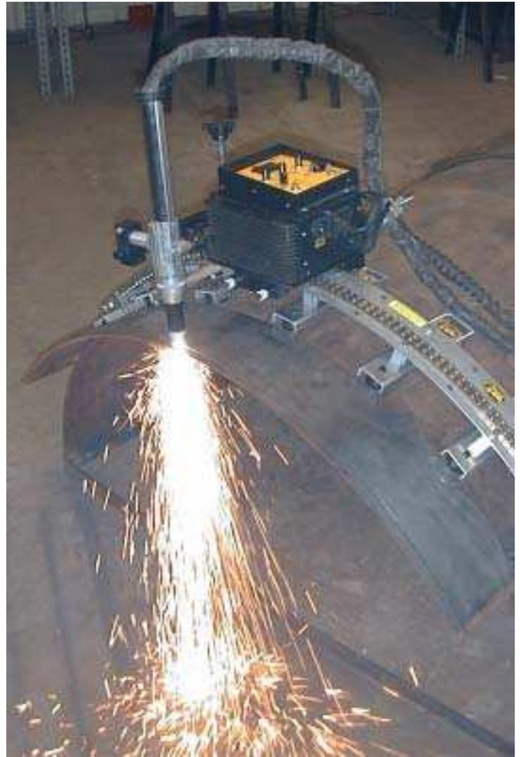
The modular design allows the user to quickly reconfigure the unit for straight line cutting or welding, stitch welding or weave welding, all with the same machine!
