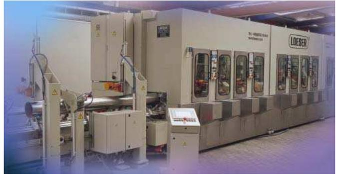
The pressure controlled grinding combined with grinding to size for screwed cylinders of up to 16m length reduce a 2 step operation to one single pass operation in a single machine. Tremendous production increase with reduced handling is the result.
