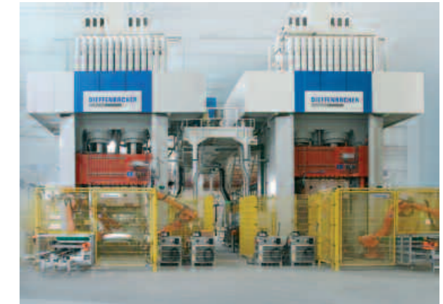
Fully automated SMC press line
