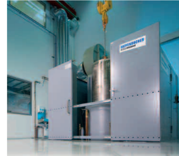
HIP machine for manufacturing highly compressed ceramic components such as artificial hip joints
