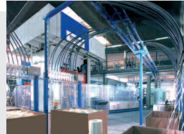
LFT-D line for manufacturing fiber-reinforced automotive parts
